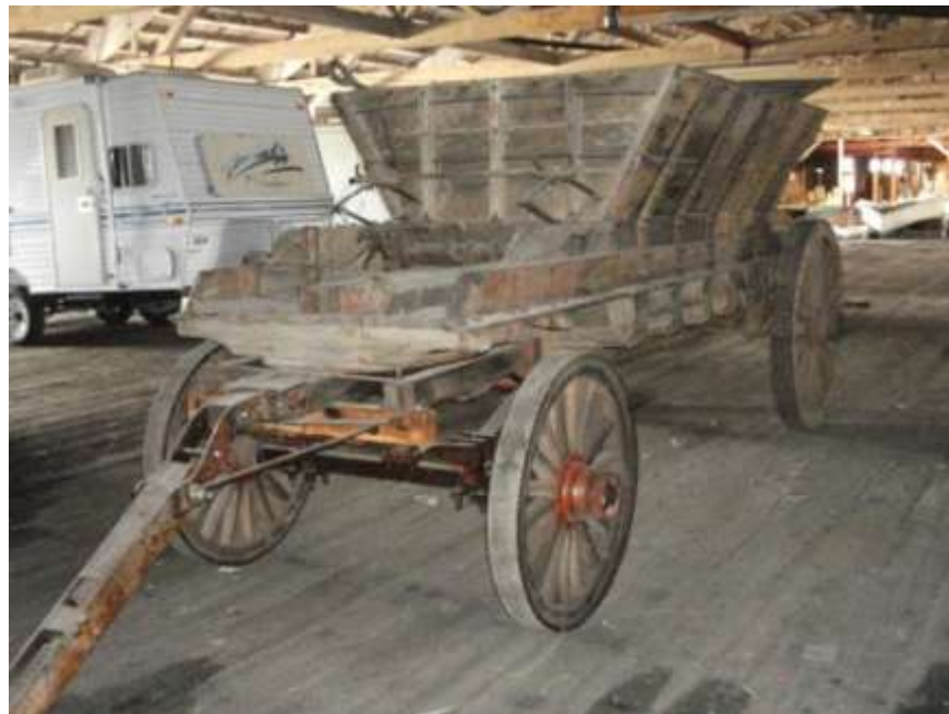
Horse drawn belly dump buckboard Used by road crews in the late 1800's or early 1900's Mint condition
